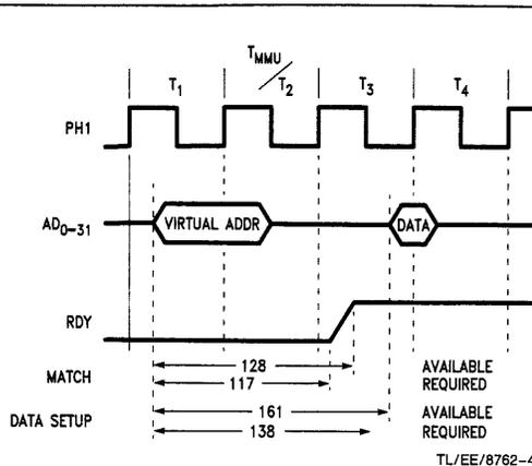
**FIGURE 4. NS32332 Cache Read. The protocol at 15 MHz is designed to drive realistic cache memory without wait states.**
