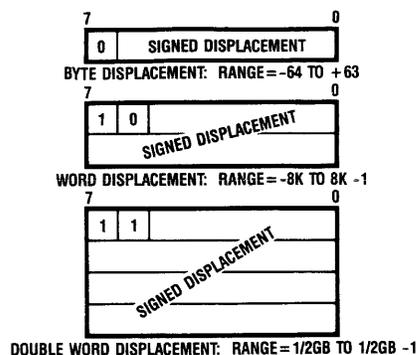
Figure 2-3. Displacement Encodings
