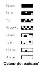
This means that, as a Mode 2 screen is 160 pixels by 256 pixels, we will dump 960 (=6\*160) by 512 (=2\*256) dots on the printer.
