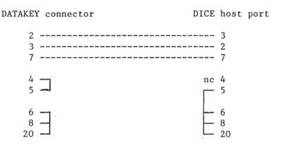
It has been found that this cable works with most DICE/PC combinations. In case of difficulty, check with your system documentation that pin 2 is transmit data. If not, connections 2 and 3 should be reversed in the above diagram.
